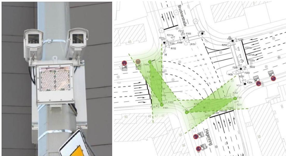
Figure 3: Single pole installation of SENV (left) and bird's eye view of all sensor locations (right).
