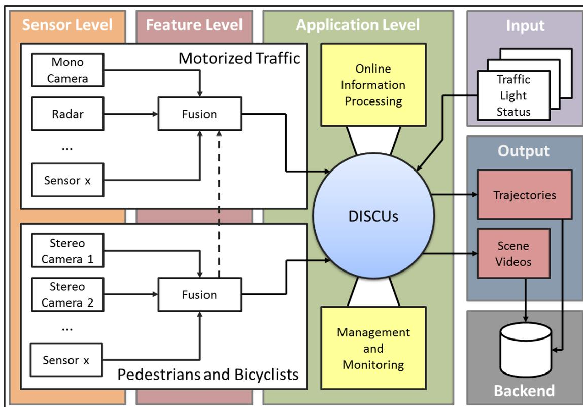
Figure 1: Functional architecture of AIM Research Intersection.
