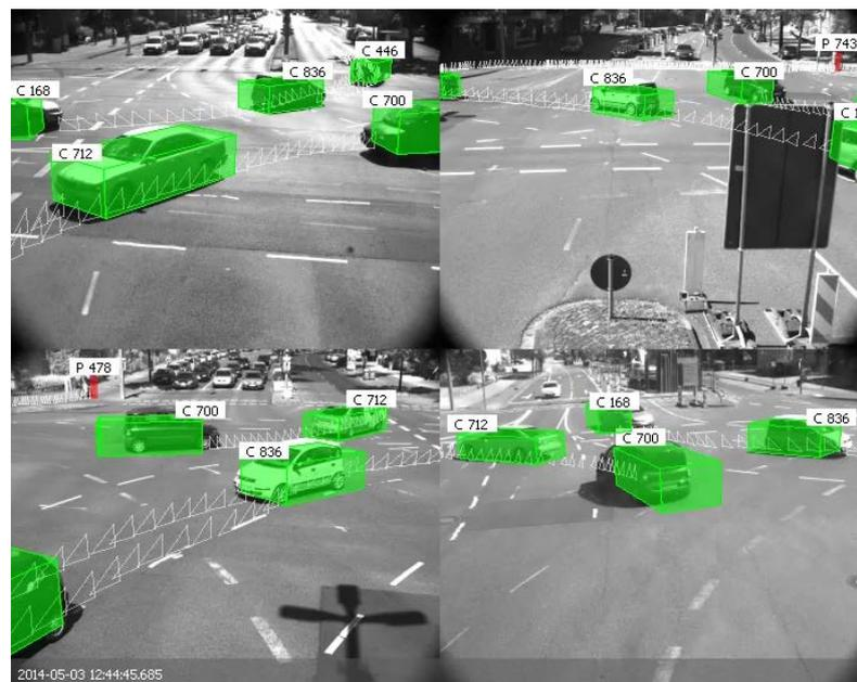
Figure 4: Visualization of a given traffic scene from the four MSS perspectives with augmented object information.
