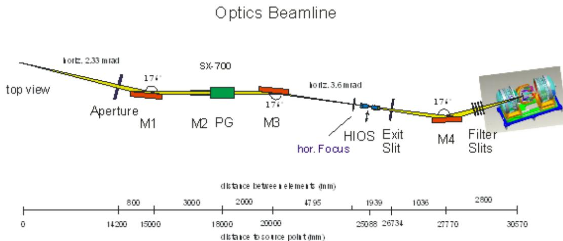
Figure 1: Optical layout of beamline PM-1 with Reflectometer end station
