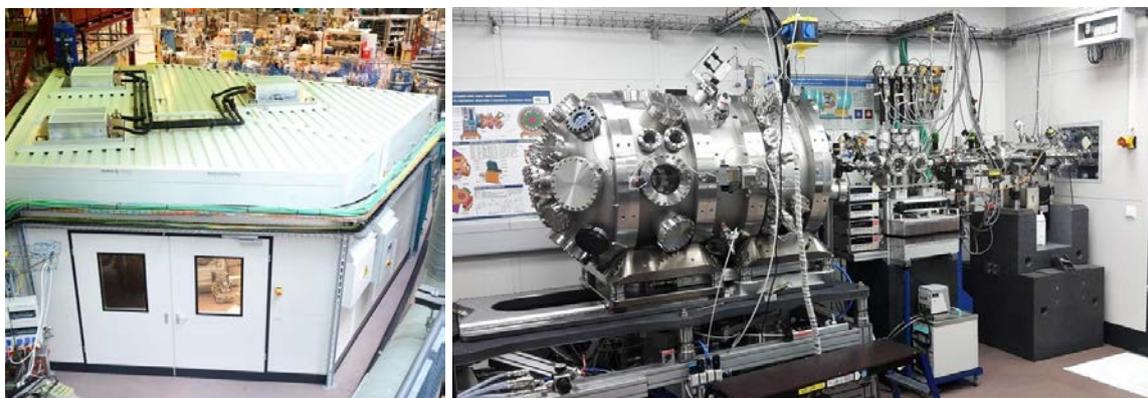
Figure 3: The clean-room hutch at the experimental floor of BESSY-II with the M4-mirror chamber, the Filter and Slit Unit (FSU) and the Reflectometer inside (Light comes from the right side).
