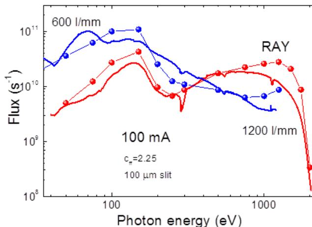
Figure 2: Photon flux at the sample position in the reflectometer, normalized to 100 mA ring current (blue (600 l/mm) and red curve (1200 l/mm)), in comparison with raytrace calculation with RAY (points). Typically BESSY-II runs with 300 mA.
