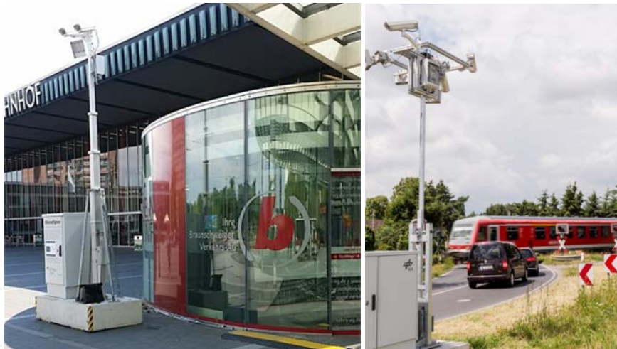
Figure 2: Mobile sensor poles at railway station and level crossing.
