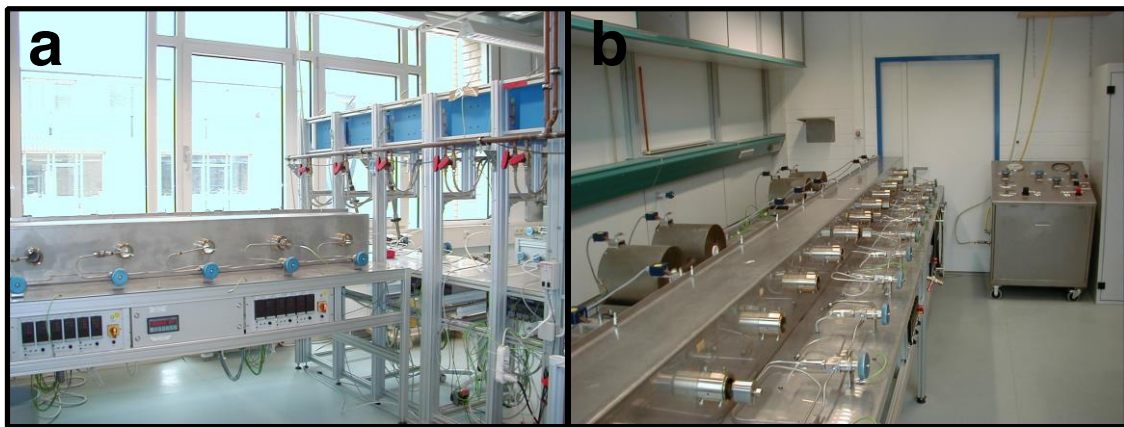
Figure 1: a) 200 MPa line and rapid quench line, b) 500 MPa line.
