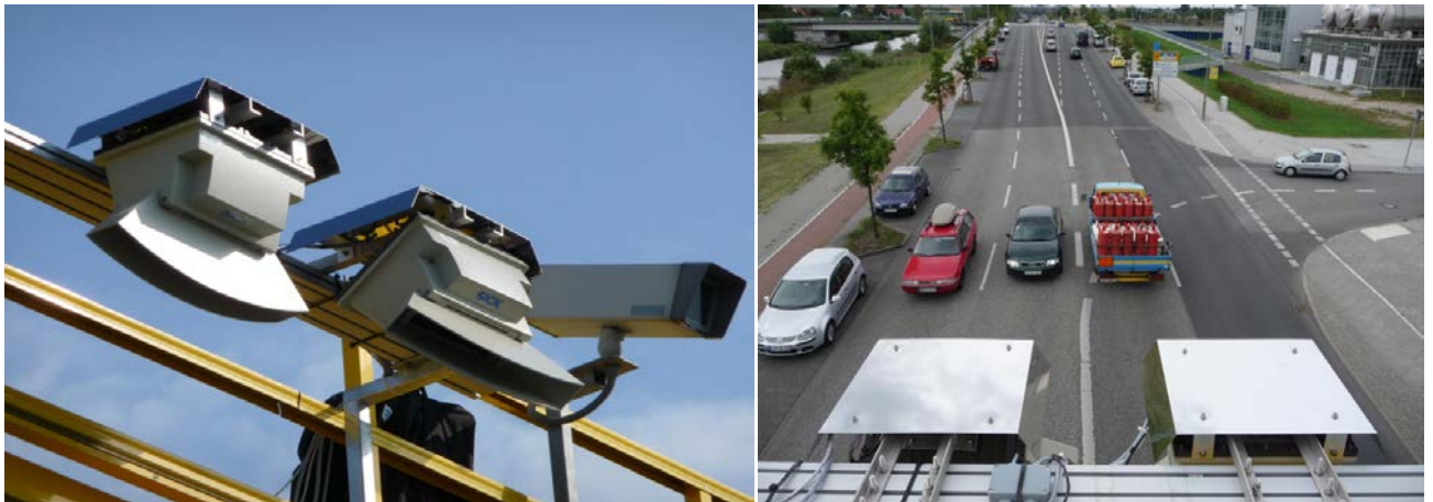
Figure 5: Profiling laser scanners.
