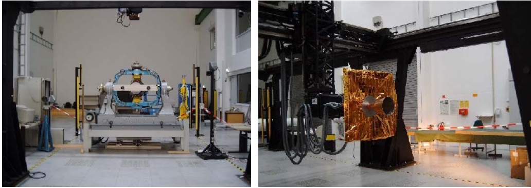
Figure 1: The former EPOS 1.0 facility: a fixed part (left) and a movable part (right)
