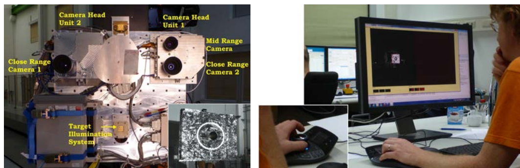
Figure 20: VIBANASS sensor system (left) and operator-in-the-loop (right).
