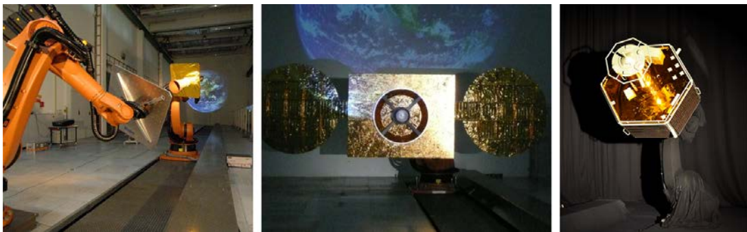
Figure 2: EPOS 2.0 facility - Physical part of the facility showing robots from different views and with different mockups and background. Left: two robots representing satellites in close proximity, center: large mockup with two antennas with a projection of the Earth in the background, right: large 3D mockup on a robot with black molton wrapping and with black background
