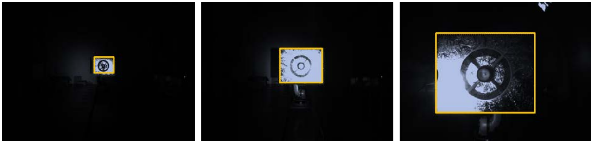
Figure 16: Examples of camera images captured with a Prosilica GC-655M showing a client satellite mockup in the laboratory at different distances. The detected edges are marked with orange color.
