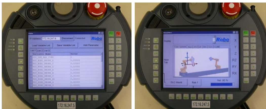
Figure 9: Manual Control Unit (MCU) - Numerical Display Window (left) and Graphical Visualization (right)
