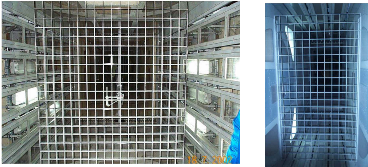
Figure 5 – Main and secondary IWT test section icing grid (Esposito et al., 2003; Ragni et al., 2005)
