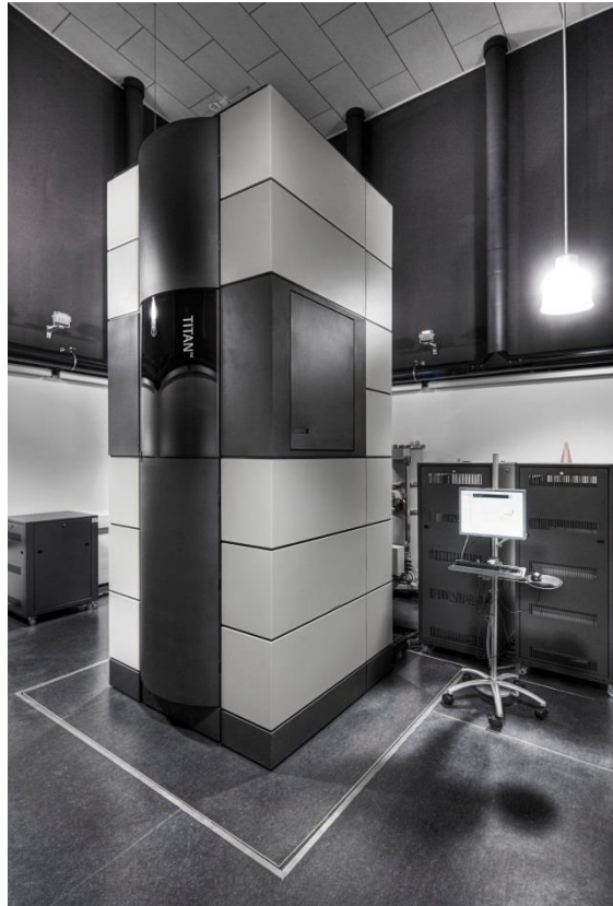
Figure 1: FEI Titan G3 50-300 PICO transmission electron microscope (photograph by courtesy of Christian Lüning ( www.arbeitsblende.de )).
